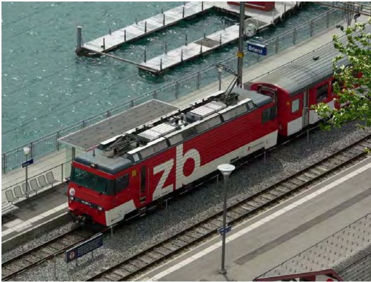
Swiss private operator Zentralbahn's, 1000mm gauge HGe 101 electric locomotive 101966 arriving at Brienz station on 18th July 2008 with a train for Luzern. (Robert Brown)
